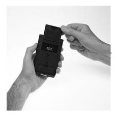
If the program does not launch, re-insert the module. Once the module is installed, turn your PDA on and tap the *PDR2000* icon.
